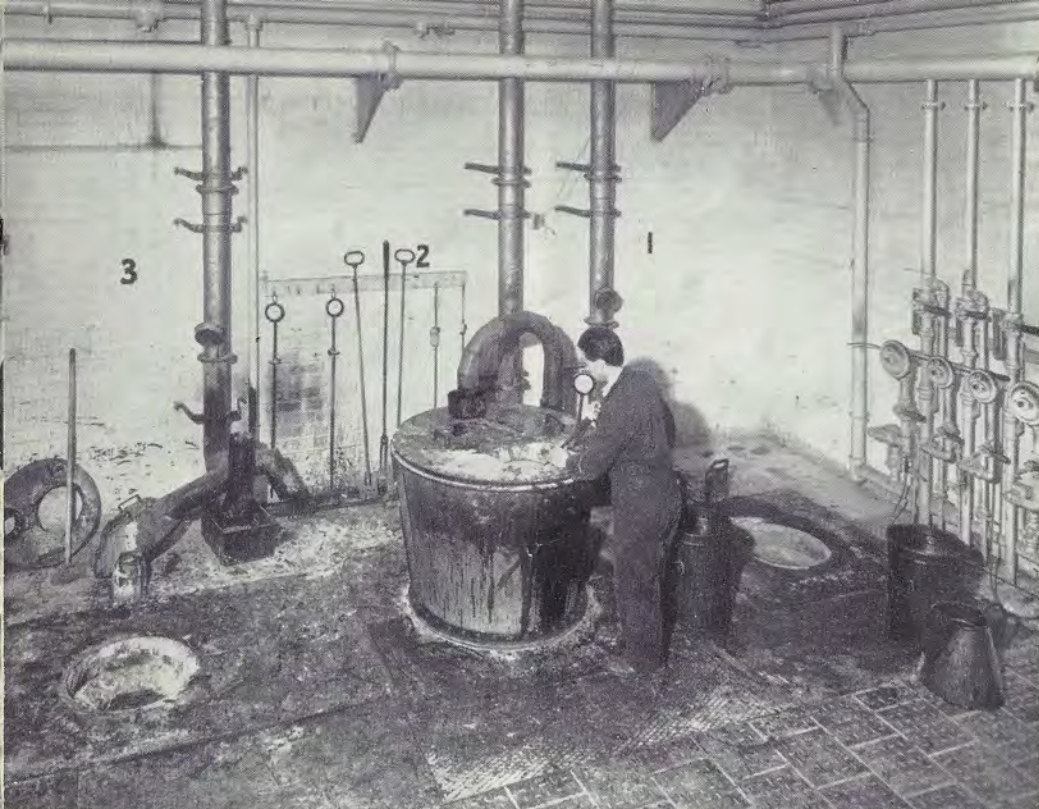
Varnish-making the old way. The resin was stirred in this type of cauldron, heated by gas jets sunk into the floor.
